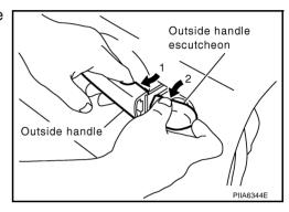
6. While pulling outside handle, slide toward rear of vehicle to remove outside handle.
