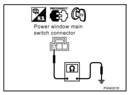
Check continuity between power window sub-switch (front passenger side) (door lock and unlock switch) connector D36 terminal 11 and ground.
