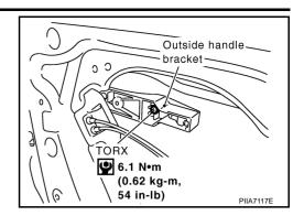
While pulling outside handle bracket, slide toward front of vehicle to remove outside handle bracket.
