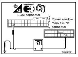
Check continuity between BCM connector M3 terminal 22 and front power window switch (door lock and unlock switch) connector D36 terminal 16.
