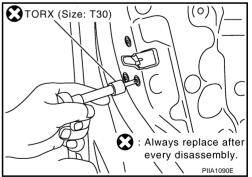
14. Disconnect the door lock actuator connector and remove door lock assembly.
