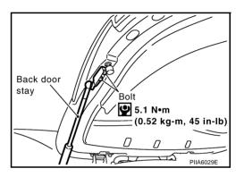
3. Remove back door stay assembly on vehicle.
