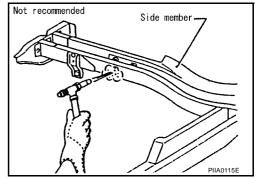
When straightening body panels, use caution in pulling any HSS panel. Because HSS is very strong, pulling may cause deformation in adjacent portions of the body. In this case, increase the number of measuring points, and carefully pull the HSS panel.
