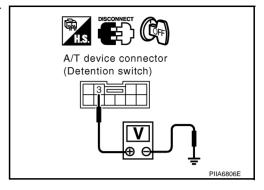
Check continuity between A/T device (detention switch) connector M67 terminals 3 (R/Y) and ground. (Check harness for short.)
