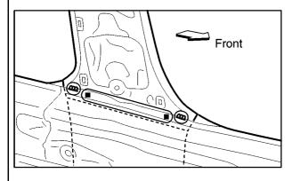
Position inner center pillar service part as overlapped old part, then M.I.G seam and plug weld.
