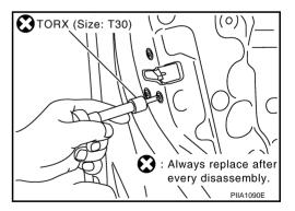
12. Disconnect the door lock actuator connector and remove door lock assembly.
