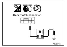
4. Check continuity between back door switch connector D109 terminal 7 and ground. (Check harness for short.)
