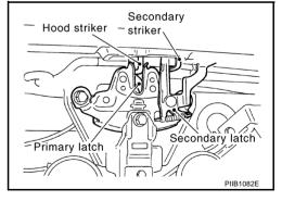
3. When pulling hood opener lever gently, make sure that front end of the hood rises by approximately 20 mm (0.79 in) and that hood striker and hood lock primary latch are disengaged. Also make sure that hood opener returns to the original position.
